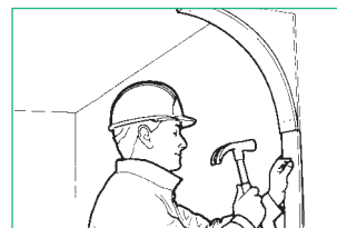
3. Position the Plaster Arch in the partition corner and screw to timber studding. Taking care to align the arch. Do not over-tighten screws.
