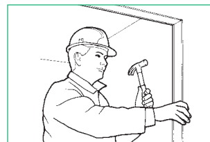
1. Corner of stud partition ready to receive Plaster Arch.
